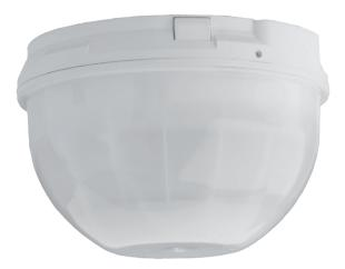
The ceiling mount panoramic DS9360 TriTech® PIR/ Microwave Detector uses several patented processing techniques to provide excellent catch performance with freedom from false alarm. Supervised microwave and PIR sections ensure that the detector is working properly. Field replaceable mirrored optics allows it to be mounted on ceilings from 2.5 m to 6 m (8 ft to 18 ft) in height.
