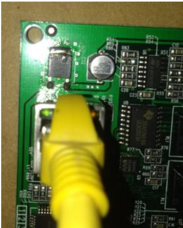
FIGURE 7 – Comnav Ethernet Port Connection.
