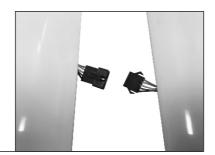
1. Place the 3 panels on the table and connect plugs on both sides.
