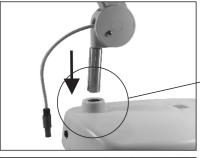
3. Insert metal rod into base panel.
