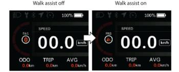
The walk assist mode is limited to 6km. Release the button "-" to stop the walk assist mode
