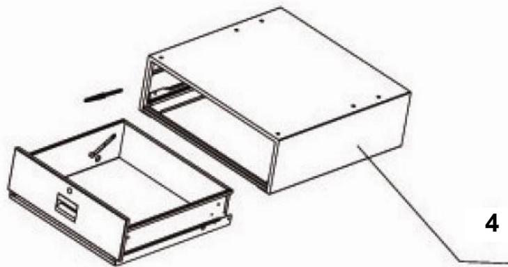
3. Attach the **Fixed Mounts (A & B)** to the **Drawer Shell (4)** with Bolts, and then carefully insert Drawer into the Shell.
