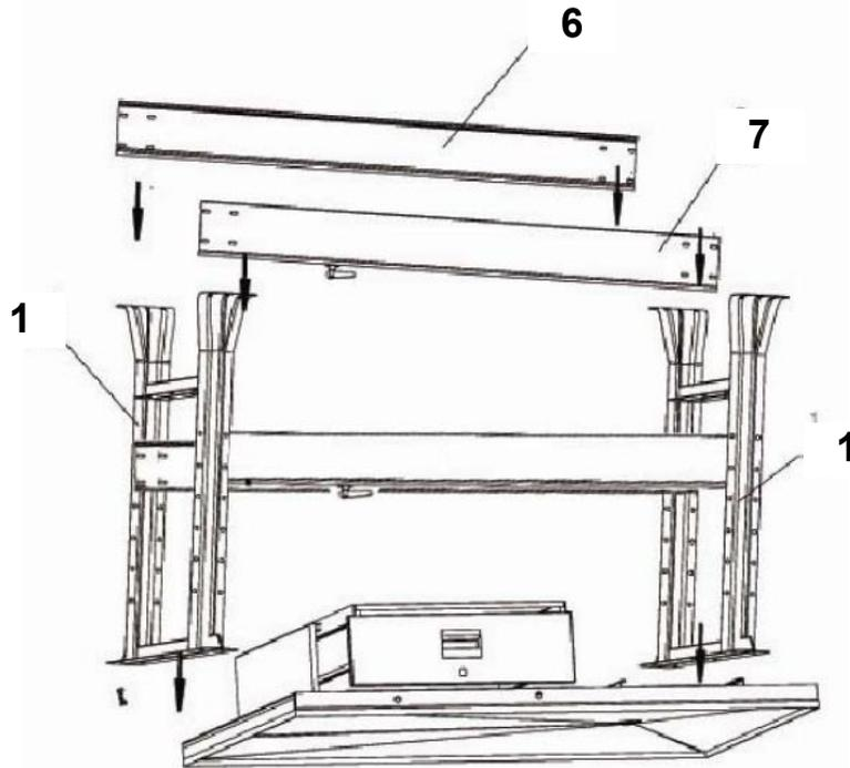
6. Carefully rotate the assembled **Table** with **Leg Assemblies (1)** and **Support Rails (6 & 7)** in the upright position.
