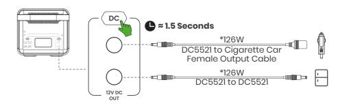
Press and hold the DC power button for 1.5 seconds until the button lights. Press and hold the button for 1.5 seconds again to turn power off to the DC ports. \*Output power total is 126W
