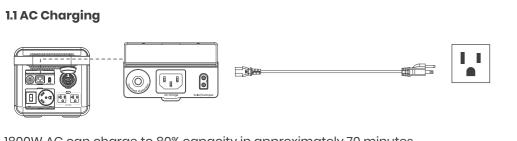
1800W AC can charge to 80% capacity in approximately 70 minutes.
