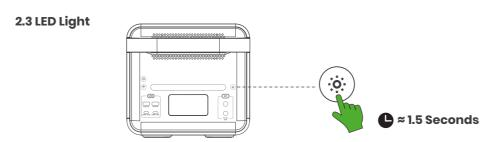
Press and hold the LED Light Button for 1.5 seconds until the LED light turns on. Press and hold the button for 1.5 seconds again to turn the LED light off.
