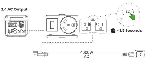
Press and hold the AC Power Button for 1.5 seconds until the button lights. Press and hold the button for 1.5 seconds again to turn off power to the AC outlets.
