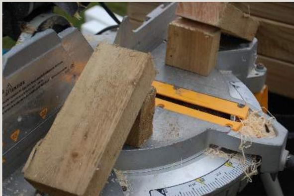
Cut 2 blocks/pieces of timber to the measurement you made a note of, be sure they are square. Now cut 2 slightly longer lengths as per the the image to form an “L” shape and screw together.
