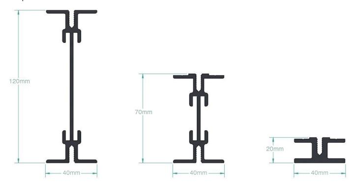
Synergised aluminium decking is a complete decking system, with one of the most advanced, high strength sub-frame systems available on the market. The subframe is available in 3 standard heights (120, 70 & 20mm) to cover all your requirements, and all joist options are the same width (40mm), and use the same unique fixing system, which dramatically cuts down on-site installation time.
