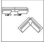
To form clean, attractive corners, the Bottom Channel can be notched with snips (see figure 3) and then bent to the desired angle. (Attached to the ground as shown in figure 4).
