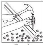
Attach the Bottom Channel component directly to the ground through the pre-punched holes (*see figure 2*). Spikes are required every 24 inches, extra holes are provided in the Bottom Channel component for convenience. Another spike or drift punch may be used to drive spikes in completely. To allow for expansion, leave a ½" gap between each section of the Bottom Channel component.
