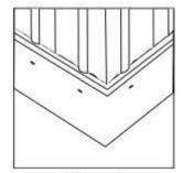
The Top Trim Back component is installed by driving the fasteners in the middle of every slot (see figure 5). *Do not fasten tightly !* (See fastening instructions on front page.) **Do not cut Top Trim Back components at the corners**. Gently bend over a sharp edge of a cutting table or a similar surface to form a corner (see figure 6).
