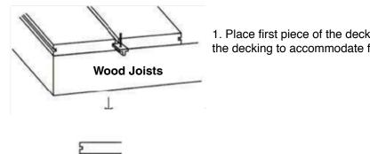
1. Place first piece of the decking at the edge perpendicular to the wood joist. Notch the decking to accommodate for the 100 x 100mm Post.
