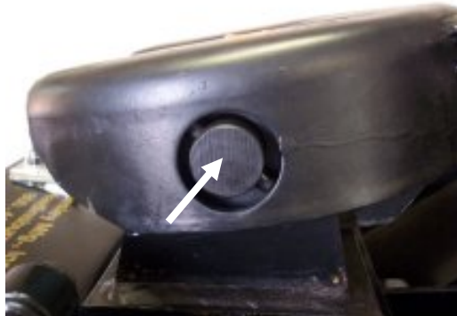
Figure 8.1 Lubricate fore and aft pivot pins
