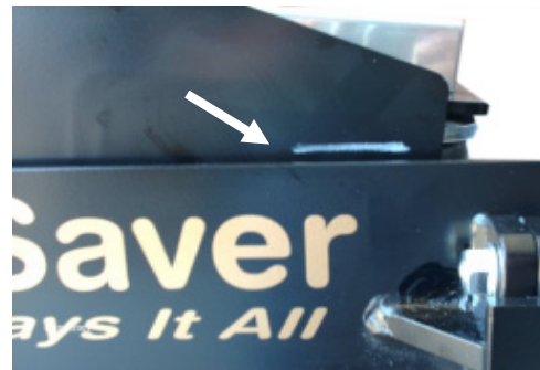
Figure 4.6 Inflating to the white mark
