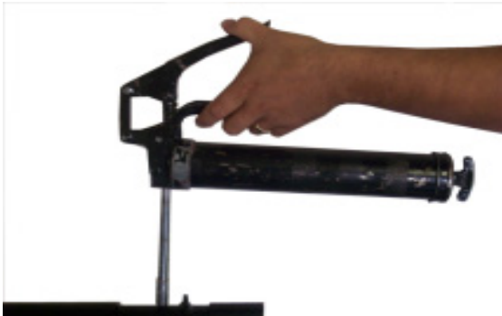
Figure 7.1 Grease every 4,000 miles
