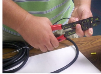
Figure 4.16 Strip ¼" insulation
