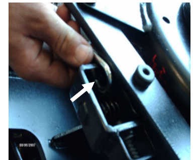
Figure 5.7 Padlock into Eight o'clock position
