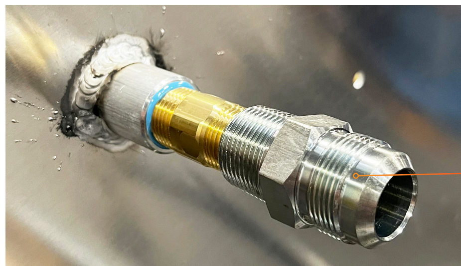
Photo 17: Attaching the Male Flare Hose Adapter
