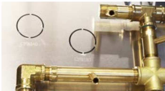
Photo 1: Pilot Assembly Knockouts
