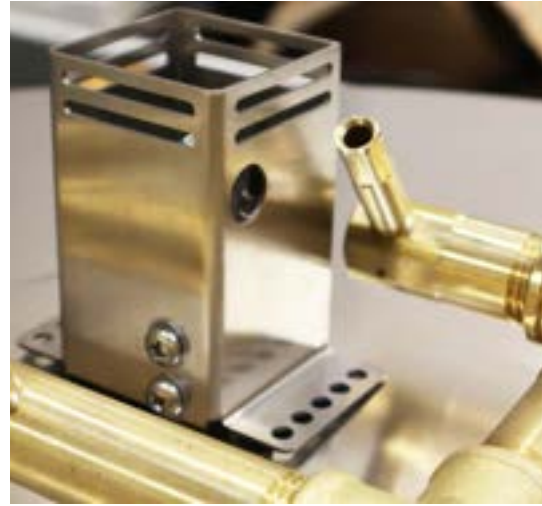
Photo 4b: Pilot Hood Circular Opening Positioning
