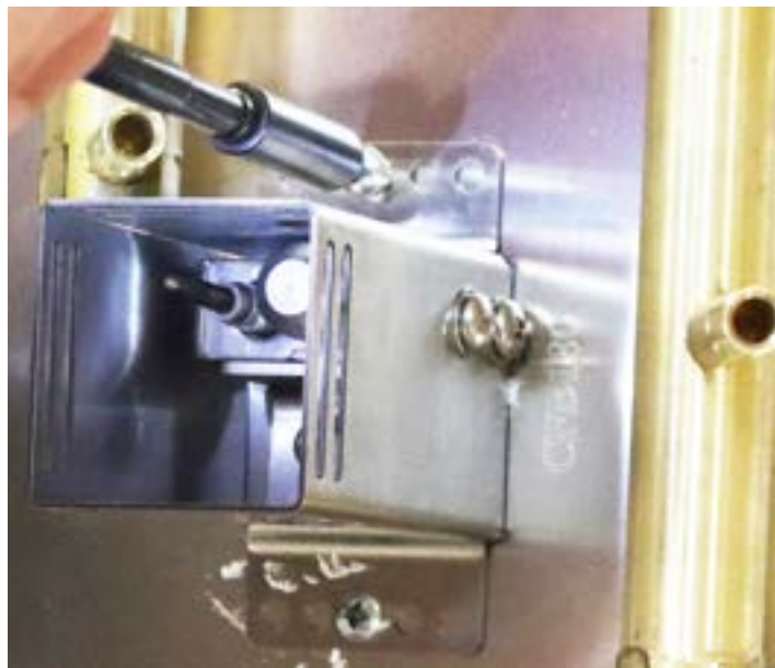
Photo 5: Securing the Pilot to the Plate/Pan
