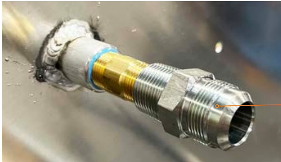
Photo 17: Attaching the Male Flare Hose Adapter
