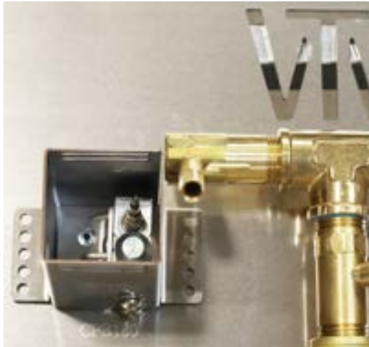
Photo 4a: Thermocouple Positioning
