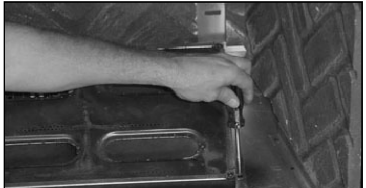
Figure 2.11 Removing Burner Support Screws
