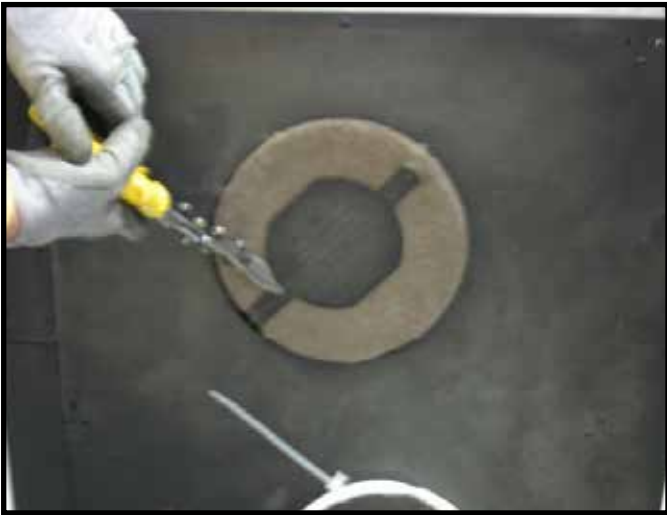
Figure 6.6 Cut the metal retaining band.
