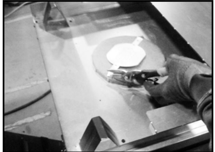
Figure 6.3 Cut the metal retaining band and fold the sides out.
