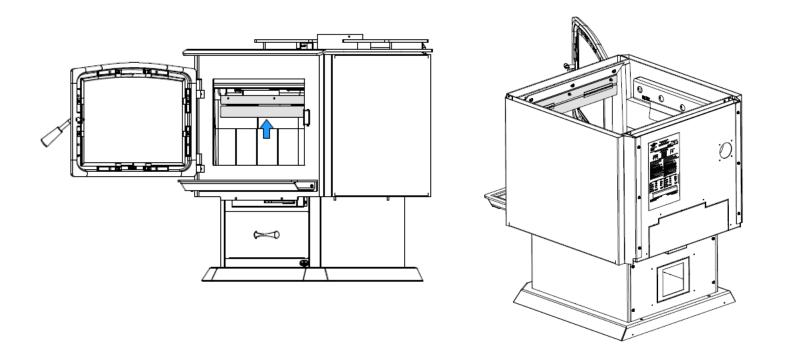
3. Hold the fire screen by the two handles and bring it close to the door opening.
