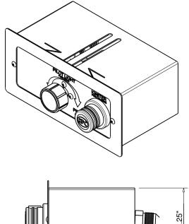
SPARK IGNITION BY AA BATTERY MATERIAL: 304 STAINLESS STEEL
