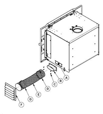
Then, install the fresh air kit adapter (B) using 4 screws (C). Secure the flexible pipe<sup>1</sup> (E) to the adapter (B) using one of the adjustable pipe clamps (D). Secure the other end of the pipe to the outside wall termination (F) using the second adjustable pipe clamp (D). The outside wall termination (F) must be installed outside of the building.
