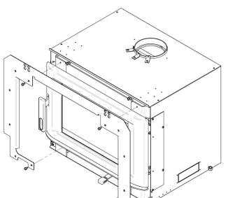
2. Put together the steel face plate with the two parts of the cast iron faceplate.
