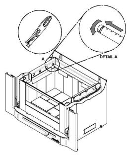
Align the notch in the left end of the tube with the key of the left air channel hole. Using a « Wise grip » hold the tube and lock it in place by turning the tube as shown in DETAIL A. Make sure the notch reaches the end of the key way.
