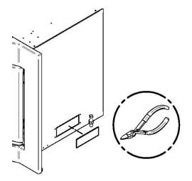
Using pliers, remove the rectangular knockout plate (A) located on the left or right side of the convection air jacket. Choose the side that is best for your installation.
