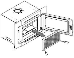
Hold the fire screen by the two handles and bring it close to the door opening.
