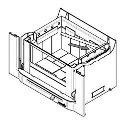
Starting with the rear tube, lean and insert the right end of the secondary air tube into the rear right channel hole. Then lift and insert the left end of the tube into the rear left channel.
