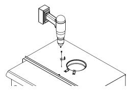
The long end of the brackets must be attached to the insert. Insert the chimney liner into the flue collar of the unit and secure the liner to the brackets with three self-tapping screws (not included).
