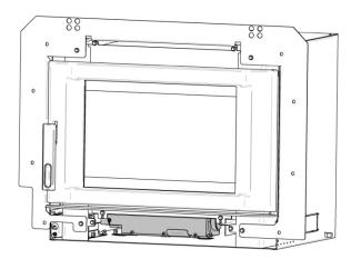
A blower is already installed on this insert. It is located underneath the insert, behind the bottom faceplate. Its function is to increase airflow through the heat exchanger and improve hot air circulation in the room. When used regularly, the blower can provide a small increase in efficiency, up to 2%. However, the use of a blower should not be used as a way to gain more output from an insert that is undersized for the space it is intended to heat.
