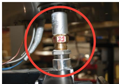
Figure 9.1 – Locating orifice for cleaning
