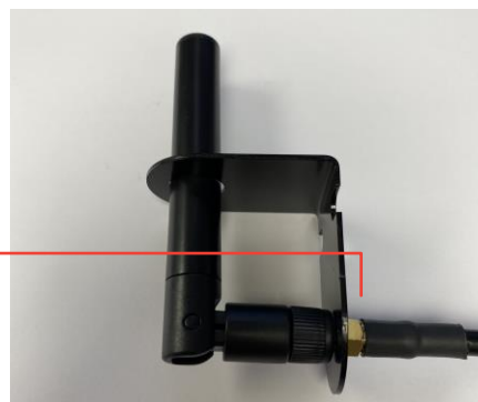
Figure 6.6 – Attach antenna cable
