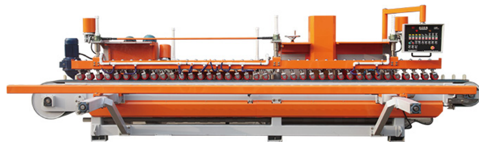
Rock plate 45° chamfering machine: straight edge and beveled edge (45°) polishing, grinding edge forming and polishing process is carried out continuously. It has the advantages of fast processing speed, high surface finish, standard straightness and low processing cost.
