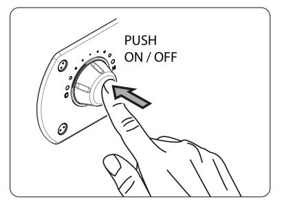
Push the wheel button once to turn on. Water flows out of outlet.
