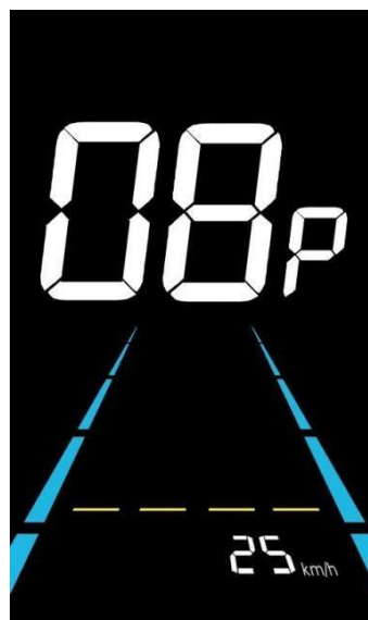
Figure 6-8 Speed limit setting interface
