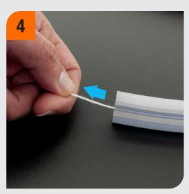
Pull the string gently, and from the other end, ensure the LED strip is not getting stuck anywhere and is moving into the channel smoothly.
