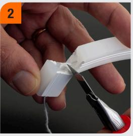
• After cutting around half of the channel, check the string inside to ensure you do not cut the string.
