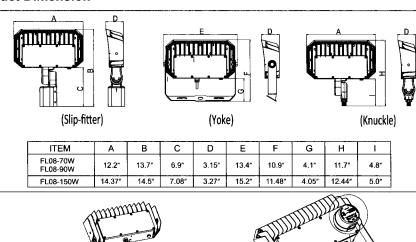
The Yoke, Slip-fitter and Knuckle can
