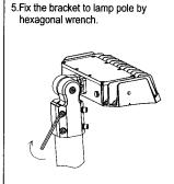
Notice: The maximum diameter of lamp pole is Ø60, lamp adjustable angle is 0-90°.
