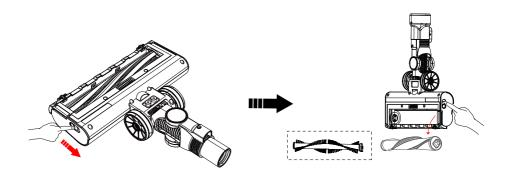
• Remove the debris wrapped around the roller with mini cleaning brush, then flush with water.
