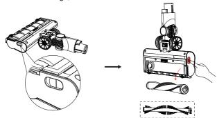
• Remove the debris wrapped around the roller with your own brush, then flush the roller with water.
