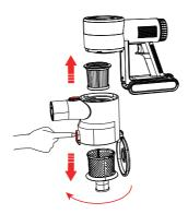
Clean the air inlet HEPA and filter cone with water.
