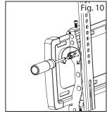
**tightened.** If you are unable loosen or fully tighten the knob by hand, the Phillips Head Screw Driver can also be used (see Fig.10).
