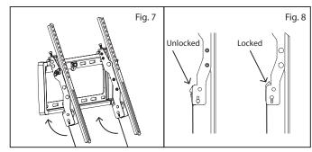
**IMPORTANT!** Verify that both arms are locked to the wall plate. For safety reasons, this mount cannot be used unless both arms are securely locked (see Fig.8)
