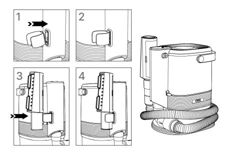
For easier use, there is another attachment to place the hose and other attachments would fit. Use the notches to clip the holder in place and have any attachment placedfor quick use.
