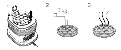
Remove the dust container and lift up the HEPA filter. Wash with water. Do not scrub, it will damage the Hepa. Drain the water as much as possible without squeezing. Once dry, place back into the vacuum with the honeycomb design facing up
