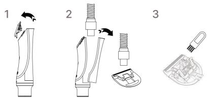
Remove the metal clippers and the cover, clean any debris on the blade and inside the attachment. Use provided brush to clean in the smaller areas.
