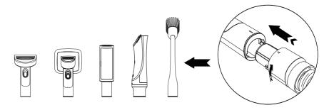
Connect the attachments by aligning and twisting to keep the attachment locked in place. Some attachments may have sharp objects, please use caution.
