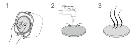
Remove the dust container and take out the foam filter. Wash with water and drain the water after cleaning. Let it set in a well-ventilated place for at least 24 hours and place it back under the dust container. Replace when needed.
