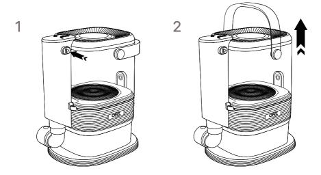
Hold the handle firmly, press the release button with your thumb, lift up and away.
