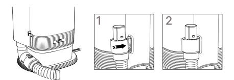
The hose can attach to the side of the vacuum using the notches to hold it in place.
