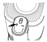
Using the Power button, turn on the vacuum. The "+" and the "-" buttons change the intensity of the vacuum.
