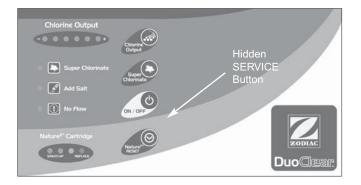
3. Continue to hold down the SERVICE button until the correct number of flashes for the controller being used is observed. Then release the button.
