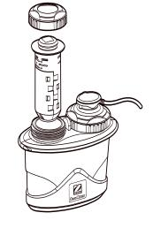
When switched on for the first time, the DuoClear will go through an initialization sequence, indicated by the yellow light being illuminated. After a short period the light will switch off and the system will begin normal operation.
