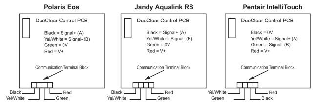
**Note**: The wiring configurations are the same for Jandy Rev K and Rev L controllers.
