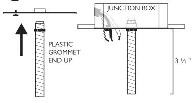
TIGHTEN LOCK NUT AGAINST FIXING STRAP TO SECURE 3 ½ " TUBE POSITION ATTACH FIXING STRAP TO JUNCTION BOX WITH JUNCTION BOX SCREWS
