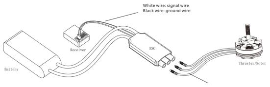
Motor ABC three-phase line, connected to ESC ABC, if the steering is not the expected steering, any two lines in ABC can be connected interchangeably to achieve the opposite of the original steering.
