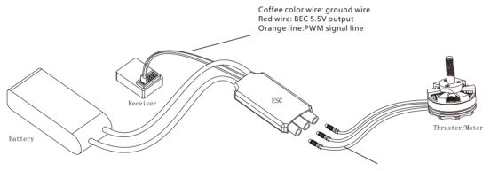
Motor ABC three-phase line, connected to ESC ABC, if the steering is not the expected steering, any two lines in ABC can be connected interchangeably to achieve the opposite of the original steering.
