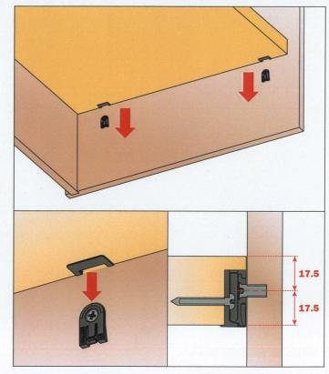
2. Drill the shelf with a  $\emptyset$  32 mm hole. Insert the shelf support in the hole and fix with WOOD screws TC  $\emptyset$  4 x 30 Z.B.
