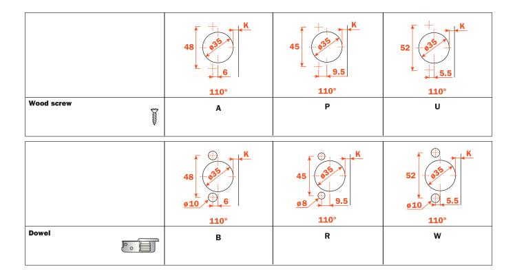
Use this table to identify the available drillings and fixings. Fill the third position of the hinge code number with the letter or the number corresponding to your choice. I.e.: CB\_2A99.
