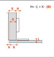
**1)** The hinge plate must be attached to the glass door with a specific adhesive using the correct procedure. We recommend that this operation is carried out by a specialist company. For further information on adhesives and their application, please contact the adhesive manufacturer or your glass supplier.
