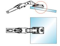
3) Rotate the cam to secure the hinge to the plate.
