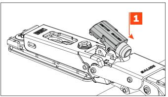
Press lightly on the back to fix in position.
