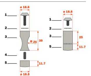
The profiles can be surface-mounted or recessed into wall systems. Screws for the profile fixing to be ordered separately. Please see page 27.
