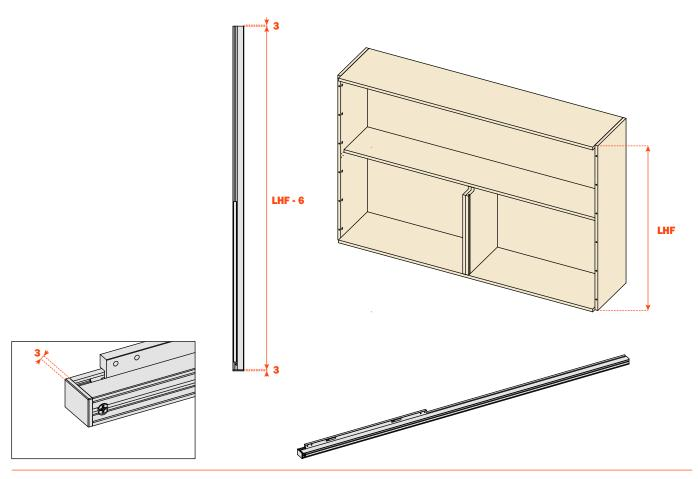
Fix the supports for the system to the cabinet sides and fix the provided cam sets.
