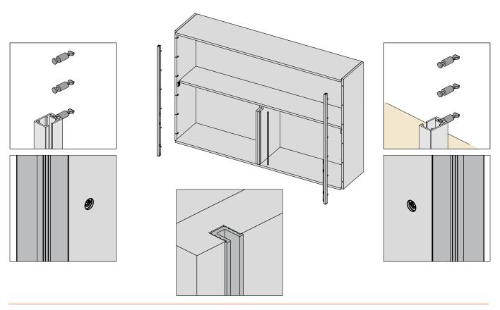
Fix the system to the supports with the screws provided.
