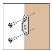
Push the door down gently until the hooks are fully engaged. When the door is in the correct position, it can be fixed to the carrier brackets with the screws provided.
