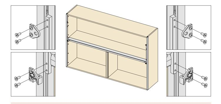
Fix the four hooks to the inside of the door with the woodscrews of the appropriate length. Hang the door onto the inner profile by locating the four hooks into their respective slots.
