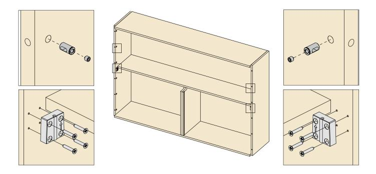
Insert the tie rods into the runners and fix them to the cabinet sides through the previously fixed cams. Fix the sliding profile to the centre panel (1800mm and 2400mm versions only).
