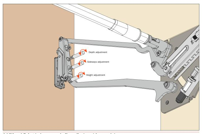
Additional fixing to be secured after adjustment is complete.
