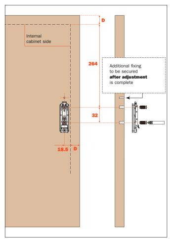
Drilling pattern for wooden door. For doors from 440 mm to 600 mm height.
