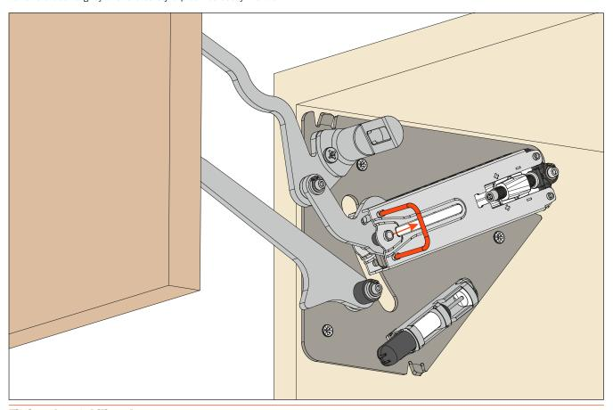
Fitting the stabiliser bar.
