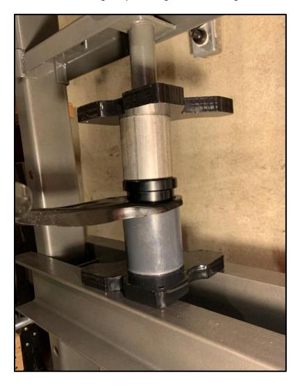
Press the bearings in from the outboard, rounded edge side of the trailing arms until they are fully seated. The bearings are fully seated when the snap ring groove is fully past the trailing arm on the inboard side.
