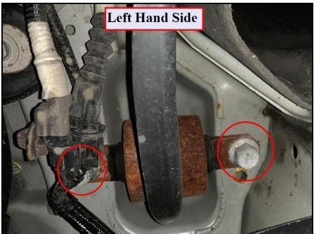
• 2.5: Remove both rear trailing arms from the vehicle. Be careful not to damage or pull the electrical wire when moving the trailing arm away from the vehicle chassis.
