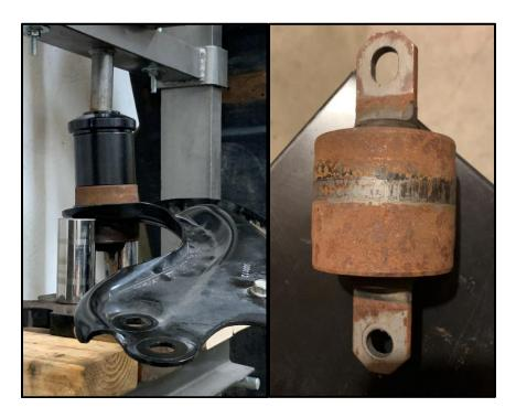
It is highly recommended to source properly sized adapters or pipe sections to brace components when in the press. During the removal of the OEM bushing using the setup shown above a suitably sized adapter was not able to be located and as such two smaller adapters were used to brace the control arm on two sides while the bearing was pressed out. This method did work to remove the bearings, but some small cosmetic damage was inflicted on the trailing arms from
