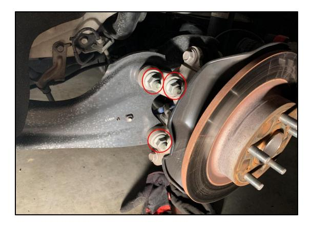
Note: After the nuts have been removed the bolts may still be difficult to remove from the joint until all 3x bolts on a given side have been loosened. Once all bolts have been loosened the trailing arm can be adjusted to remove any pressure on the bolts in order to remove them.
