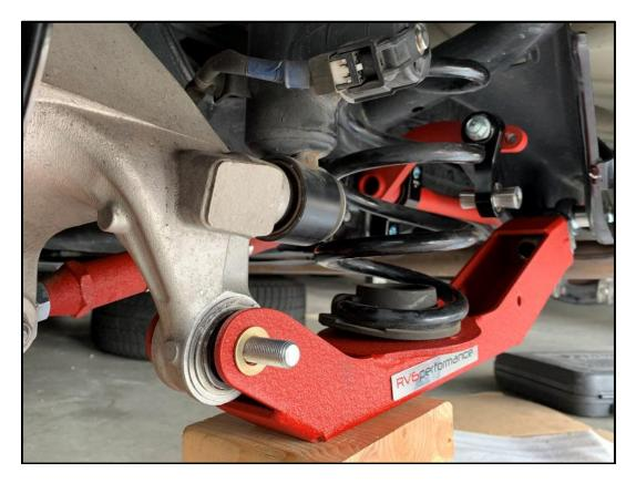
The rear knuckles may require some slight manipulation to align the mounting holes with the lower control arms. A pry bar can be used to leverage the knuckle itself until alignment is achieved. Alternatively, a pin / punch can be partially inserted into the mounting holes and used to move the components into alignment with each other so the hardware can be inserted from the opposite side of the joint. Take care to not damage any components if either of these methods are used.
