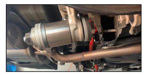
• 3.6: Place 1x of the provided shims between the rear face of the knuckle and the bearing snap ring grooves (Green Arrow) on each left and right bearing, 2x shims total. Spread 1x retaining ring with snap ring pliers and insert into the respective bearing groove to retain the shim in place (Red Arrow) on each left and right bearing, 2x retaining rings total. A flat head screwdriver can be used to help position the snap ring and ensure it is fully seated into the groove.
