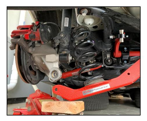
4.3: Raise the jack enough such that the upper spring caps can be correctly positioned around the retention features in the chassis on both left and right sides of the vehicle. Raise the jack slightly once the correct alignment is achieved to hold the springs in place while the outboard bolts securing the control arms to the rear knuckles are installed. See the image below.
