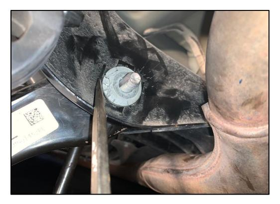
Once the washers are unthreaded from the bolts remove all components from the vehicle. This hardware will not be re-used.
