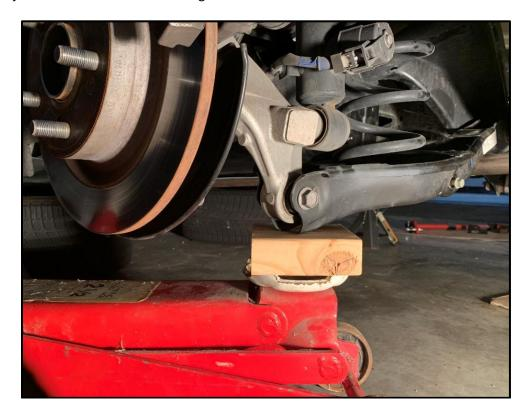
This step is required because the control arms have a load applied to them due to the suspension springs being slightly compressed in the system. Once the bolts described in Step 2.4 are removed the springs will try to release this stored energy and could cause the control arms to move forcefully and unexpectedly.
