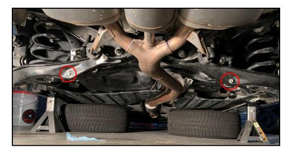
• 2.2: Position a floor jack underneath the control arms near the outboard mounting locations at the rear knuckles. It is advised to place a flat piece of scrap wood between the jack and the lower control arms to prevent damage to the painted surfaces during this process. Raise the jack until it is just starting to put pressure on the control arms but not so much that the vehicle is raised from the jack stands. Reference the image below.
