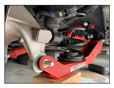
The rear knuckles may require some slight manipulation to align the mounting holes with the camber arms. A pry bar can be used to leverage the knuckle itself until alignment is achieved. Alternatively, a pin / punch can be partially inserted into the mounting holes and used to move the components into alignment with each other so the hardware can be inserted from the opposite side of the joint. Take care to not damage any components if either of these methods are used.
