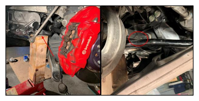
• 7.3: Manipulate the control arm and ball joint stud to allow them to assemble. Loosely thread on the castle nut (Yellow Circle.) The stabilizer link stud can also be assembled at this time by rotating the knuckle until the proper alignment is achieved. Loosely thread the flange nut onto the stud (Red Arrow.) It is advised to not connect the ride height sensor yet to prevent damage that may stem from continuing to manipulate the control arm.
