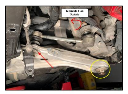
7.4: Install the rear compliance mount bearing. Locate the RV6 Performance rear compliance
