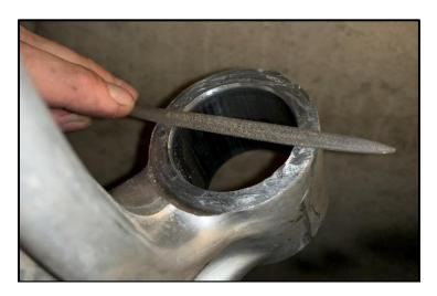
Step 6: Install the RV6 Performance spherical bearing:
