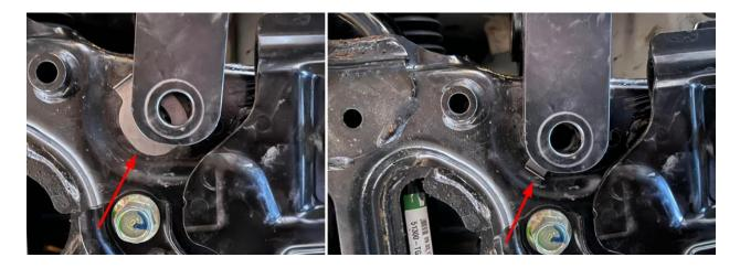
Once the housing is aligned the 1x longer bolt supplied with the kit can be loosely assembled into the inboard connection to the sub frame as shown below.
