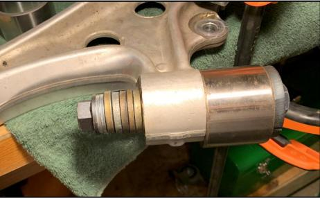
• 5.4: Prepare the control arm for the new bearings. As mentioned in the steps above a small amount of marring was incurred on the rear face of the control arm bore when prying off the integrated flange. A small file was used to remove any burrs or raised portions both on the rear face and the chamfer to the bore. The image below makes the marring look much more severe than reality due to the lighting. Small scratches on the face are acceptable as this surface only acts
