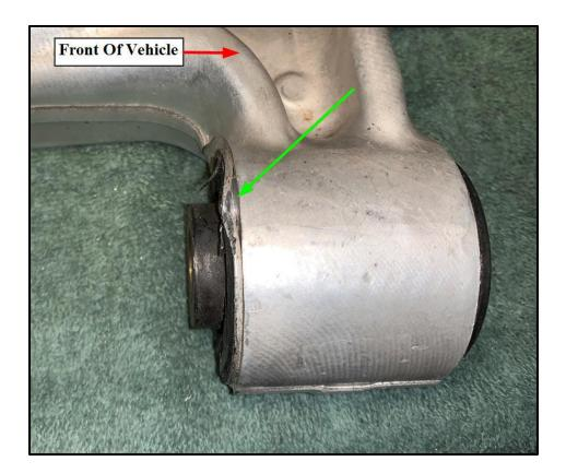
• 5.2: Prepare the bearing to be pressed out. Under normal circumstances as described in the Preface section, this step would be to brace / restrain the control arm and have a means to push the bearing out from the front towards the rear of the control arm bore. In order to setup a press for this you need 3 things: a "driver" to push the bearing, a "housing" to catch the bearing as it is pushed out, and the means to apply the force.
