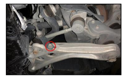
• 3.2: Remove 1x 19mm nut from the linkage stud (Red Circle.) This nut may be broken loose with a socket or impact but to fully remove the nut the stud will need to be retained with an 8mm hex bit while the nut is turned with a 19 mm wrench. See the photo below for a possible tool arrangement. Note there may not immediately be enough clearance to remove the linkage stud from the control arm - do not force the stud through the arm as this may damage the threads.
