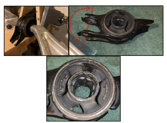
Step 5: Remove Front Control Arm Bearing:
