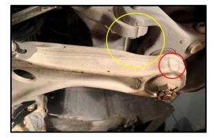
The recommendation here is to also apply a separating force to the ball joint with the use of a pry tool or a ball joint separator. A few strikes from a mallet will still be required but the force will be greatly reduced. A pry tool can be inserted between the control arm and the knuckle (area shown in Yellow Circle above) and a force can be applied to the joint while a mallet is used to strike the
