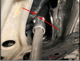
• 3.5: Remove 2x 19mm head bolts securing the rear control arm bearing / compliance mount housing to the chassis (Red Circles.)
