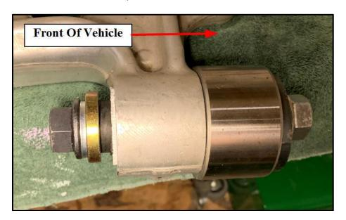
Note that the setup pictured above was intended to drive the bearing towards the front of the car, whereas the bearing should under ideal circumstances be driven towards the rear of the vehicle to be removed. This is where it is worth mentioning that there is a small but noticeable risk to performing the pressing as the images depict. As seen in an above image the integrated flange tends to shear off at a specific diameter. This diameter, while jagged from ripping the metal, is
