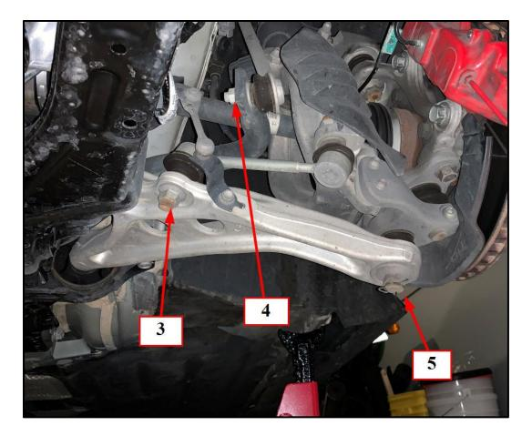
When torqueing the ball joint castle nut the recommendation would be to torque to the lower value and attempt to insert the cotter pin. If the holes in the castle nut do not align with the hole in the ball joint stud tighten the castle nut until the cotter pin can be inserted.
