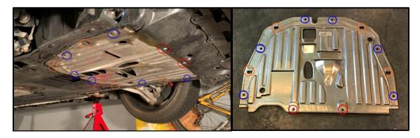
• 2.2: Remove 19x pop clips on the bottom and side faces of the plastic shrouding (Red Circles.)
