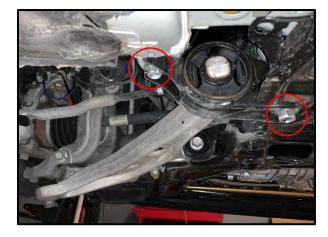
• 3.6: Using needle nose pliers remove the cotter pin from the ball joint castle nut (Red Circle.) Grasp the pin on the side profile and gently pull away from the castle nut (Red Arrow.) Once this
