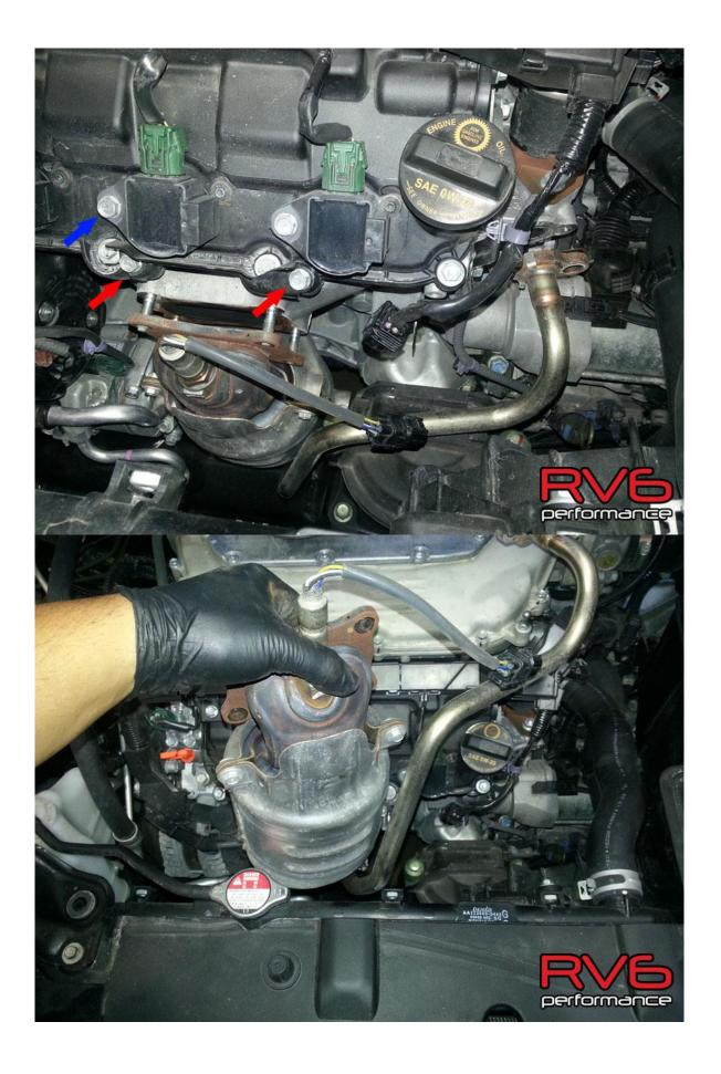
With the converter out we can compare the size of the OEM part to our RV6 PCD. With the
