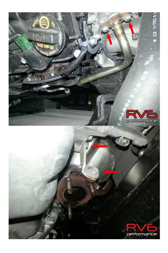
Disconnect the primary oxygen sensor clip from the harness. Remove the headshield off of the valve cover (2)10mm bolts. Remove the middle coil pack (1)10mm bolt. Once all bolts have been removed place the, aside as they will be reused for the installation of our PCD. Now slide the converter off the studs and remove the converter out of the car, be sure not to damage the radiator while removing the converter.
