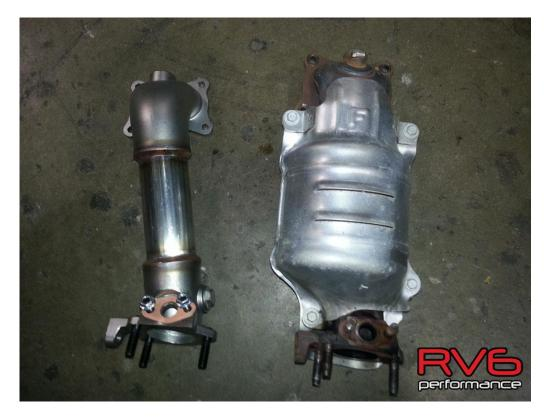
Go ahead and transfer the EGR tube over from the OEM converter to the PCD, install the new OEM exhaust gasket and reverse the order of removal to install the part. Leave all the bolts and nuts loose but snug to the engine to allow easy alignment and installation of the J-pipe.
