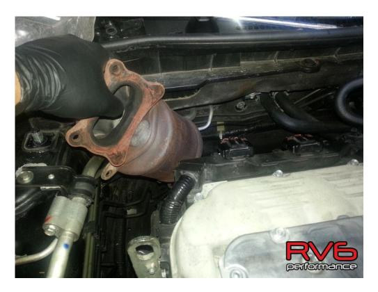
And again, you can see the difference between the OEM part and the RV6 PCD. Now reinstall the oxygen sensors into the RV6 PCD, when the part is installed on the car you will not be able to fully turn the defouler for the downstream sensor properly. (the defouler pictured is not the same as the one that will come with your EGR-B PCDS, we have extended the defouler out for this vehicle specifically to help aid in preventing and CEL from coming on.)
