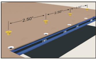
SCREW/RIVET PITCH SHOULD NOT EXCEED 2.50"
