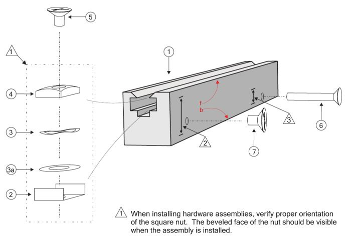
Dimension Range (#6-32 Thread): 0.150" from 'b' - 0.150" from 'f' If drilled area protrudes into the hardware slot, be sure track is clean and de-burred after tapping, and mount screw does not interfere with the hardware slot.
