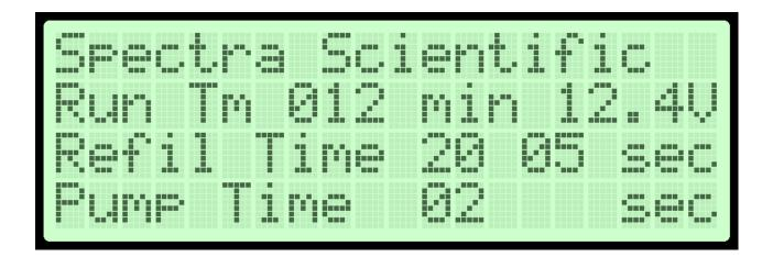
Run Time (Run Tm): This refers to the TOTAL time the controller has been ON, displayed in minutes.
