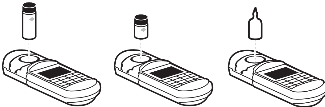
Figure 5 Placing Samples in the Sample Cell Compartment
