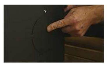
Using a screwdriver or wrench, remove the cover plate off the back of the heater.
