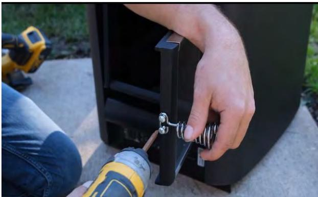
Fasten the stove handle onto the stove door With the screws provided.
