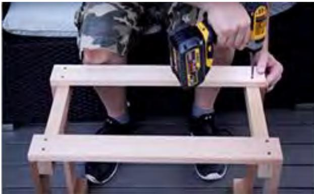
Screw heater guard support to either side using (2) – 1 ½" (38mm) screws per side.
