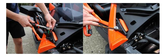
4. Starting from the rear, place the frame on the Slingshot. The two back plates go on the back headrest on the front of the roll hoop. Attach and tighten halfway with four shorter/skinnier bolts (35mm). The four long bolts (12mm) go into where the mirror brackets were. Tighten halfway on each side. Once all bolts are in place, tighten the remaining bolts. Put mirrors back on with same OEM bolts.
